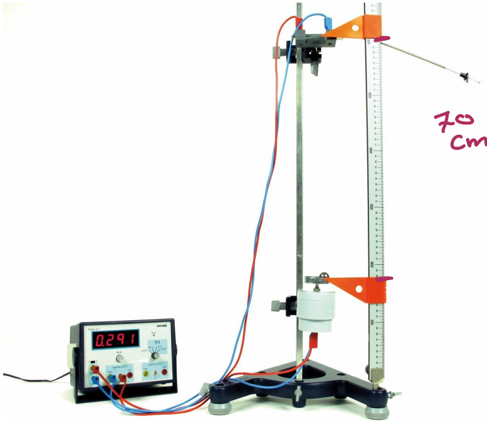
Figure: Experiment set-up for measuring the fall time of a steel ball as a function of the distance h between the trigger mechanism and a contact plate
