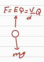
The oil drop has a mass of  $2.8 \times 10^{-14}$ kg and the distance between the plates is 1.2cm.
