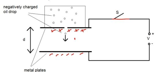
The distance between the two metal plates is d. When the switch S is closed a potential difference, V, is applied to across the plates and causes an electric field to be set up between the plates.
