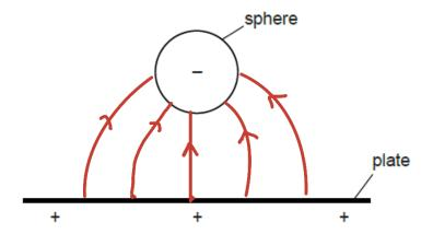
On the above figure draw **a minimum of five field lines** to show the electric field pattern between the plate and the sphere. [2]
