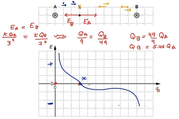
At point X, the magnitude of the resultant electric field strength due to particles A and B is zero.
