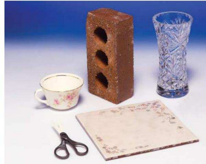
Figure 1.10 Common objects made of ceramic materials: scissors, a china teacup, a building brick, a floor tile, and a glass vase.
