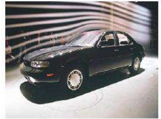
Figure3. Laminar flow around an automobile in a test wind tunnel
