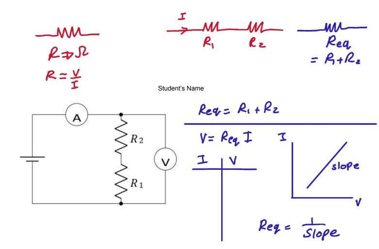
To calculate the equivalent resistance of two resistors in series
