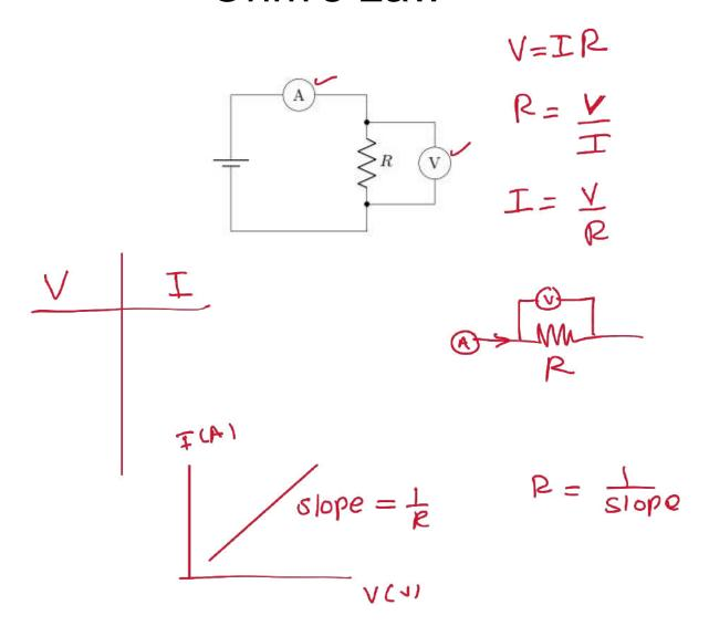
To verify Ohm's law by finding the resistance of a resistor and comparing it to its known value.
