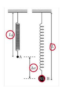
Determining the spring constant (k) by using Hooke's law.
