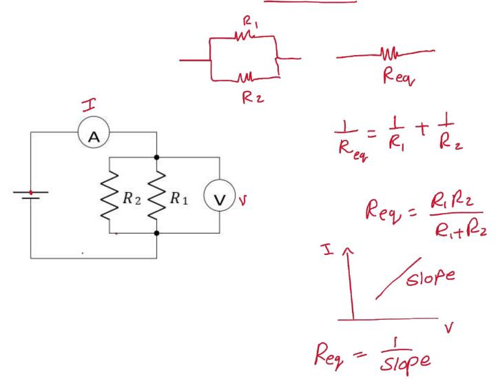
To calculate the equivalent resistance of two resistors in Parallel
