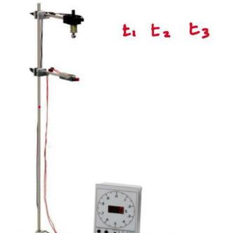
Suspend the steel ball using the holding magnet.
